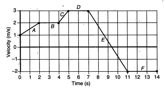
The values on the y-axis represent the *instantaneous* velocities of the object at the times marked on the x-axis. It is as though we were looking at a car's speedometer at various times. We have divided the graph into six sections: A, B, C, D, E and F. Since each section is a straight-line segment, the object's acceleration within each section is *constant*. We will learn how to interpret this graph by considering the following problem.
